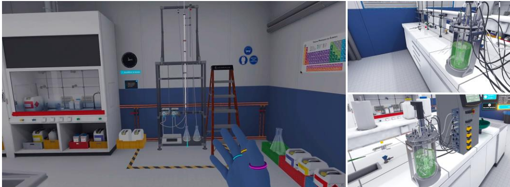
Figure 3: A liquid/liquid Extractor Pilot and a Bioreactor in the new Process Engineering Lab
