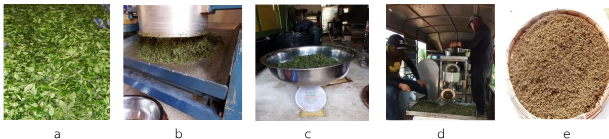
Figure 4. a. Fresh tea leaves b. Rolling tea leaves c. Tea leaves after rolling d. Tea leaves cutting e. Tea leaves after cutting
