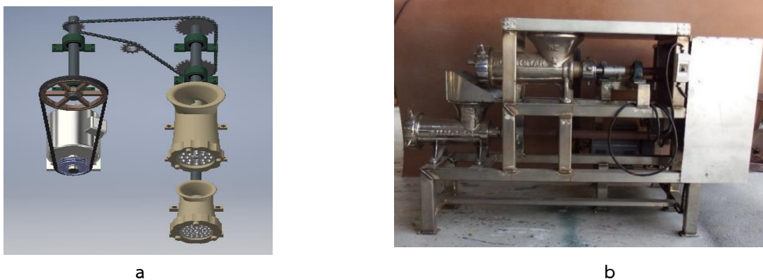
Figure 3. a. Power transmission system b. Cutting machine for black tea
