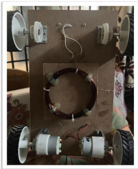
Fig4: Receiver side coiling
