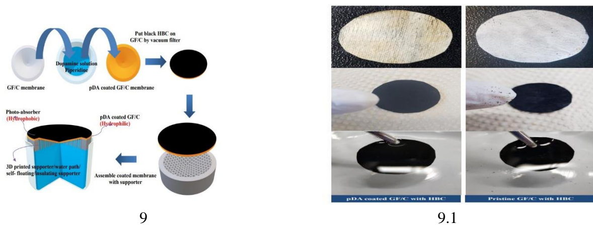
Fig.3.6 Schematic model of 3D printed solar steam generation device Fig.9.1 a)PDA coated GF/C membrane with HBC b)Pristine coated GF/C membrane with
