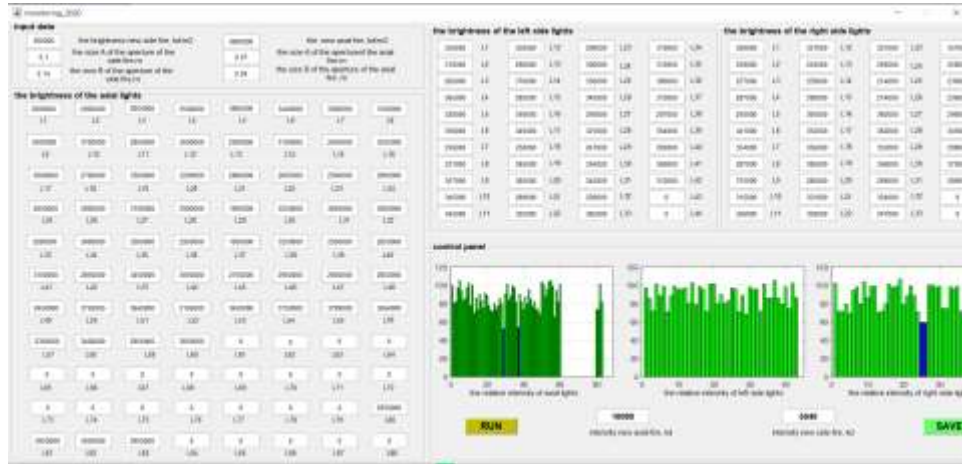
Fig. 3 Toolkit for detecting the performance of runway aerodrome lights
