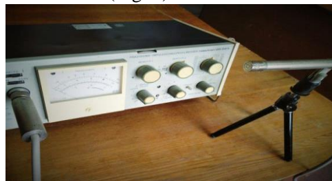
FIGURE 1. Noise recorder of the 1° class Robotron 00023 with Robotron MK 211 measuring microphone Source: author's photo
